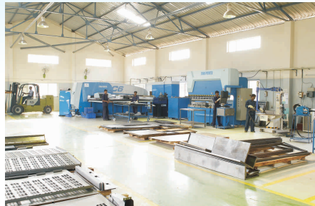
CNC Sheetmetal fabrication unit
